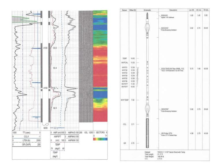
Radial Cement BOND LOG – GR – CCL – Junk Basket / Gauge Ring
